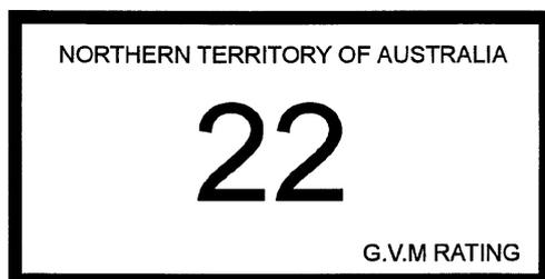
GVM rating label is placed above the GCM rating label and is applicable to the rigid vehicle or hauling unit only.
